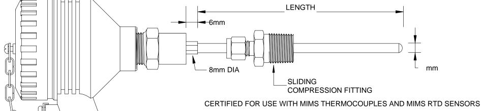
MAX 40 V 3 WATT RATING ACCEPTS 33 MM & 40 MM CENTRE TERMINAL BLOCKS OR IN HEAD TRANSMITTERS.
